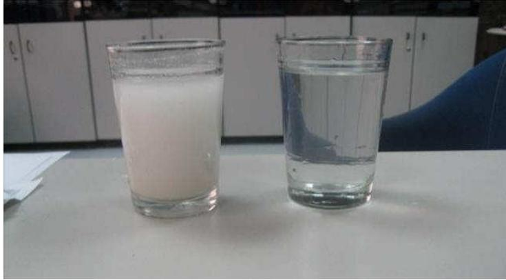
Sludge from the GRP cutting line (left) and water exiting the machine (right)
